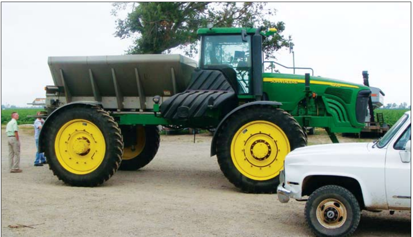
This variable-rate spreader allows for accurate field applications of fertilizers.
